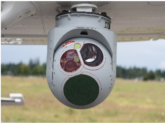
Figure 13. An MX-18 infrared camera modification underneath the aircraft. 14
